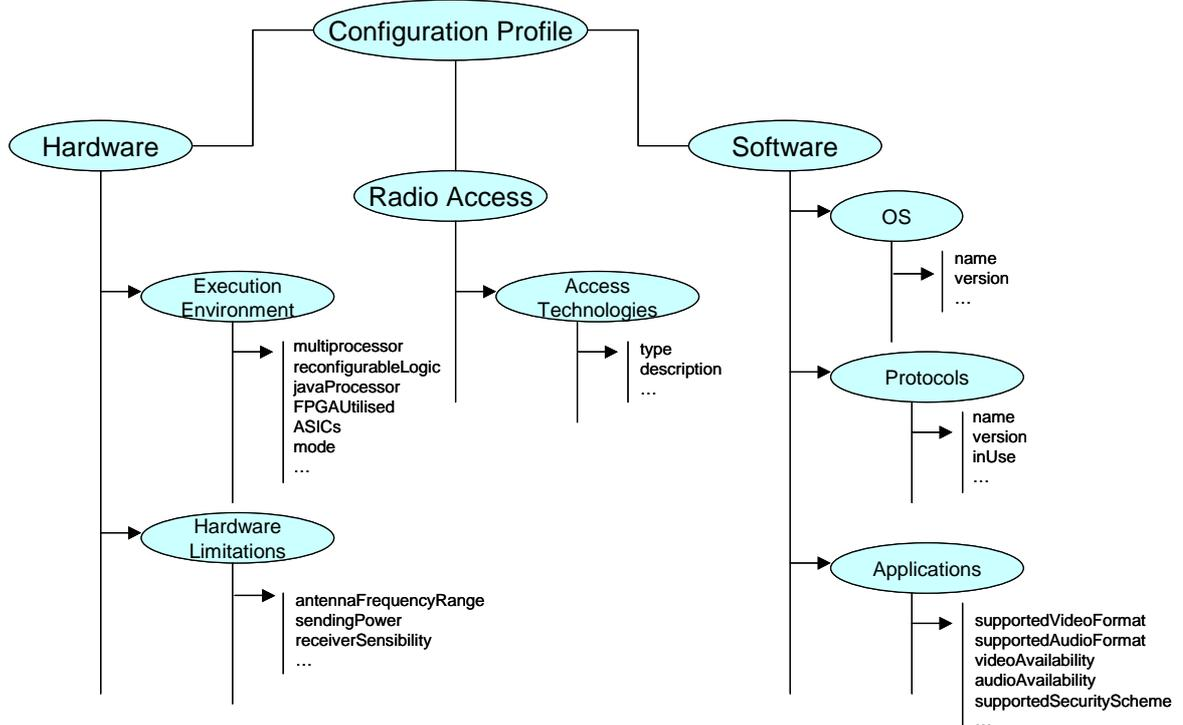
Figure 2: Terminal Configuration Profile
